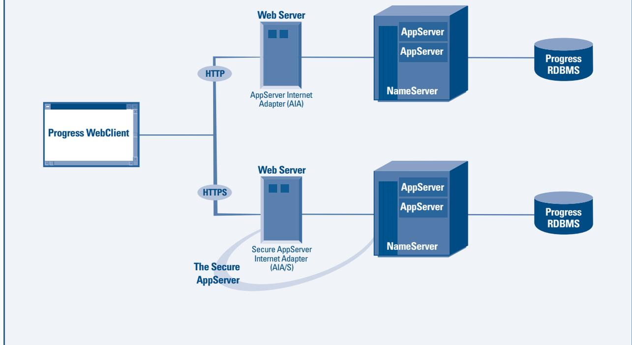
**The Progress WebClient communicates with the Progress AppServer through both HTTP and HTTPS tunneling. The Secure AppServer enables HTTPS tunneling with support for SSL encryption.**
